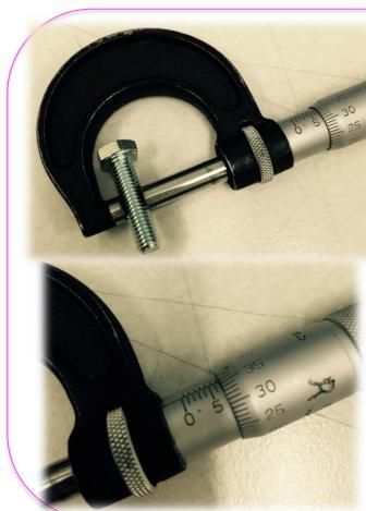
The micrometer is a precision measuring instrument, used by engineers. Each revolution of the rachet moves the spindle face 0.5mm towards the anvil face. The object to be measured is placed between the anvil face and the spindle face. The rachet is turned clockwise until the object is 'trapped' between these two surfaces and the rachet makes a 'clicking' noise. This means that the rachet cannot be tightened any more and the meas
